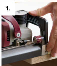
1. Mill P-System grooves in the shelves and move the centre position to the workpiece. Drill an access opening
