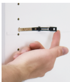
1. Mill P-System grooves in the shelves and move the centre position to the workpiece. Drill an access opening
