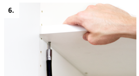
6. Tighten the Clamex P-14 Flexus
